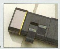
safe even when removed from the Organiser II. They are available in sizes 8K, 16K, 32K, 64K and 128K sizes and each machine can take two at a time giving as much as 320K of on-board memory in our LZ64 model.
